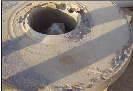
Damaged wear plate at 22 days
